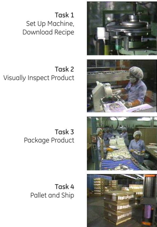
Figure 1. Mix Automated and Manual Tasks Unlike traditional systems, industrial workflow allows production teams to mix automated and manual tasks
