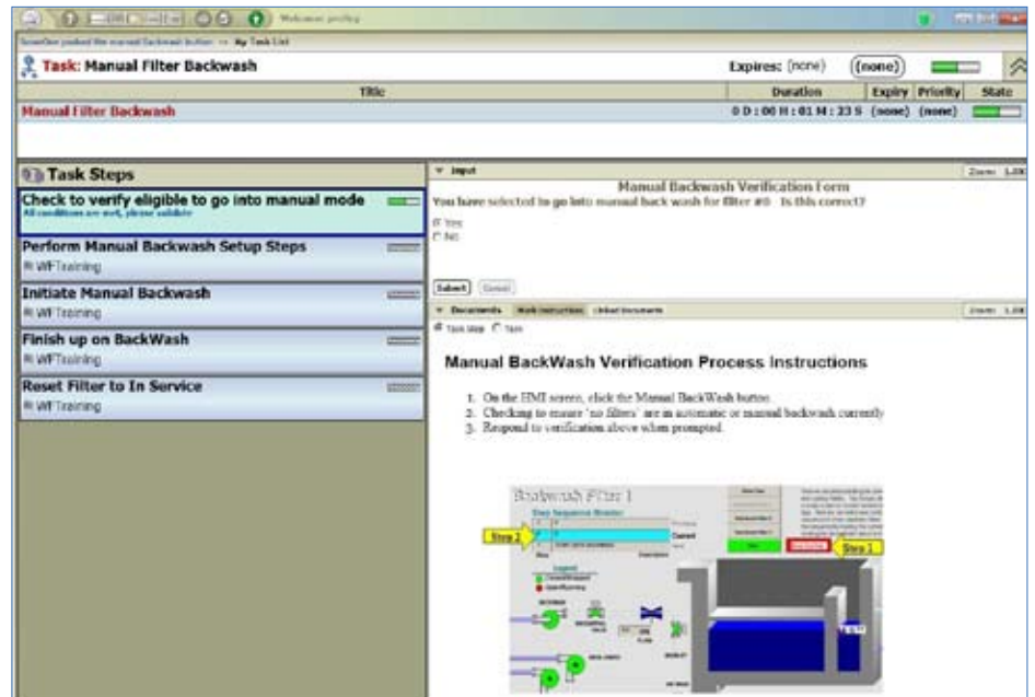
As an example of Electronic Work Instructions, Proficy Workflow can guide operators through the process of a manual filter backwash
